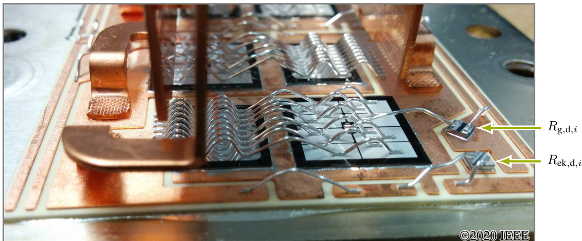
Figure 7.1: Photo of the discrete internal resistors mounted on each DCB substrate [103]
