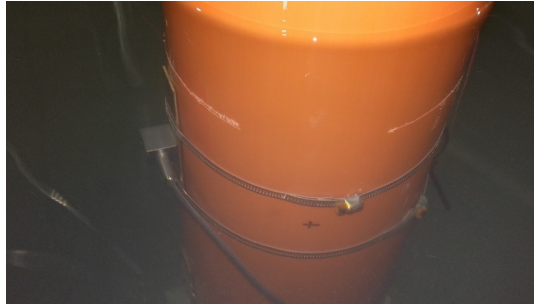
Fig. 5. Symmetrical damage application on the test structure
