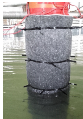
Fig. 4. Synthetic sheet used as marine growth replacement
