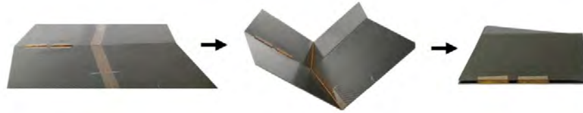
Fig. 6: Carbon Fiber prototype of a single degree-four vertex undergoing folding motion showing simplicity as a result of minimizing the structure to a single unit cell.
