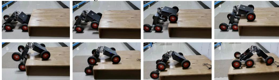
Fig. 9. The experiment of the robot climbing 200 mm vertical obstacle.
