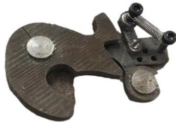
Fig. 12. Physical drawing of novel ratchet and pawl mechanism
