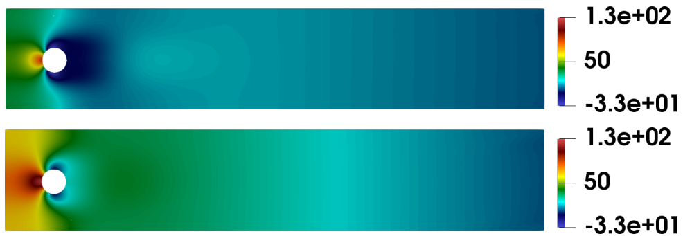
Figure 5. The pressure p for the configuration “cold to warm” (above) and “warm to cold” (below)
