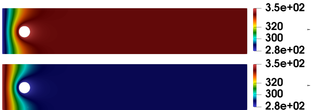
Figure 6. The temperature \vartheta for the configuration “cold to warm” (above) and “warm to cold” (below)
