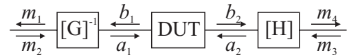
Fig. 6. Error model of a two-port VNA with four measurement channels on the basis of the 7-term model.
