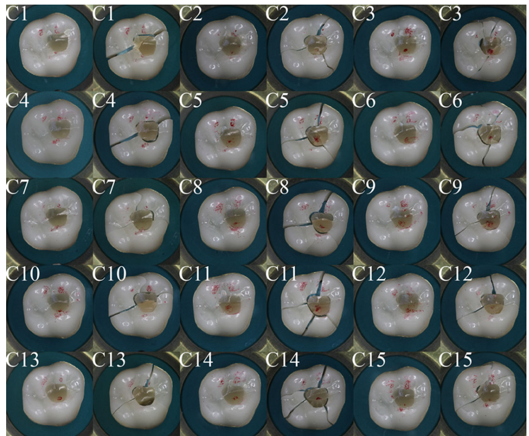
Figure 7. Crowns from group C, before and after the fracture test; the red features indicate the areas where contact with the steel ball occurred; post-fracture the remaining pieces were reconstructed.
