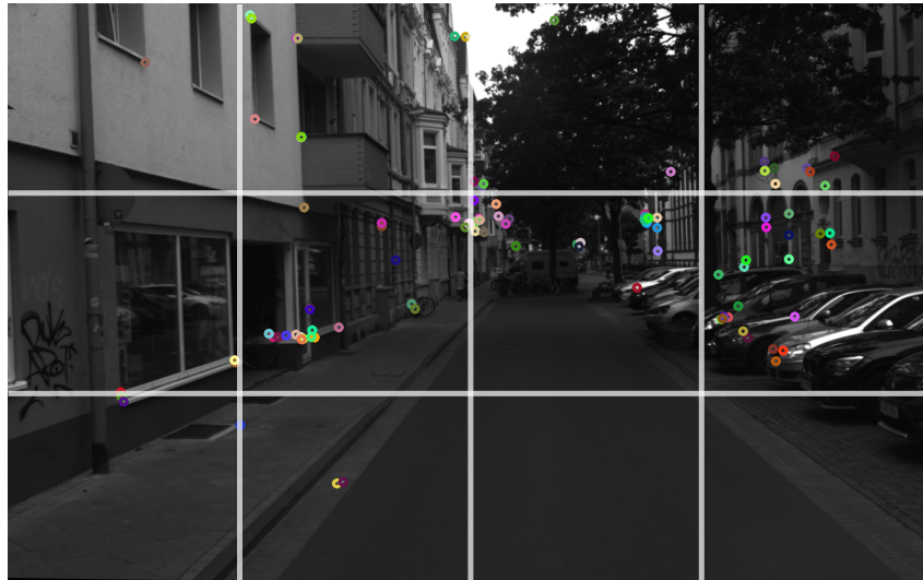
Figure 4.5: ORB-feature detection and image tiles. The detected features are colored. The image plane is divided into tiles with identical sizes in which features are detected. White lines visualize the border of the tiles. This enables to detect features that are well distributed on the image plane.
