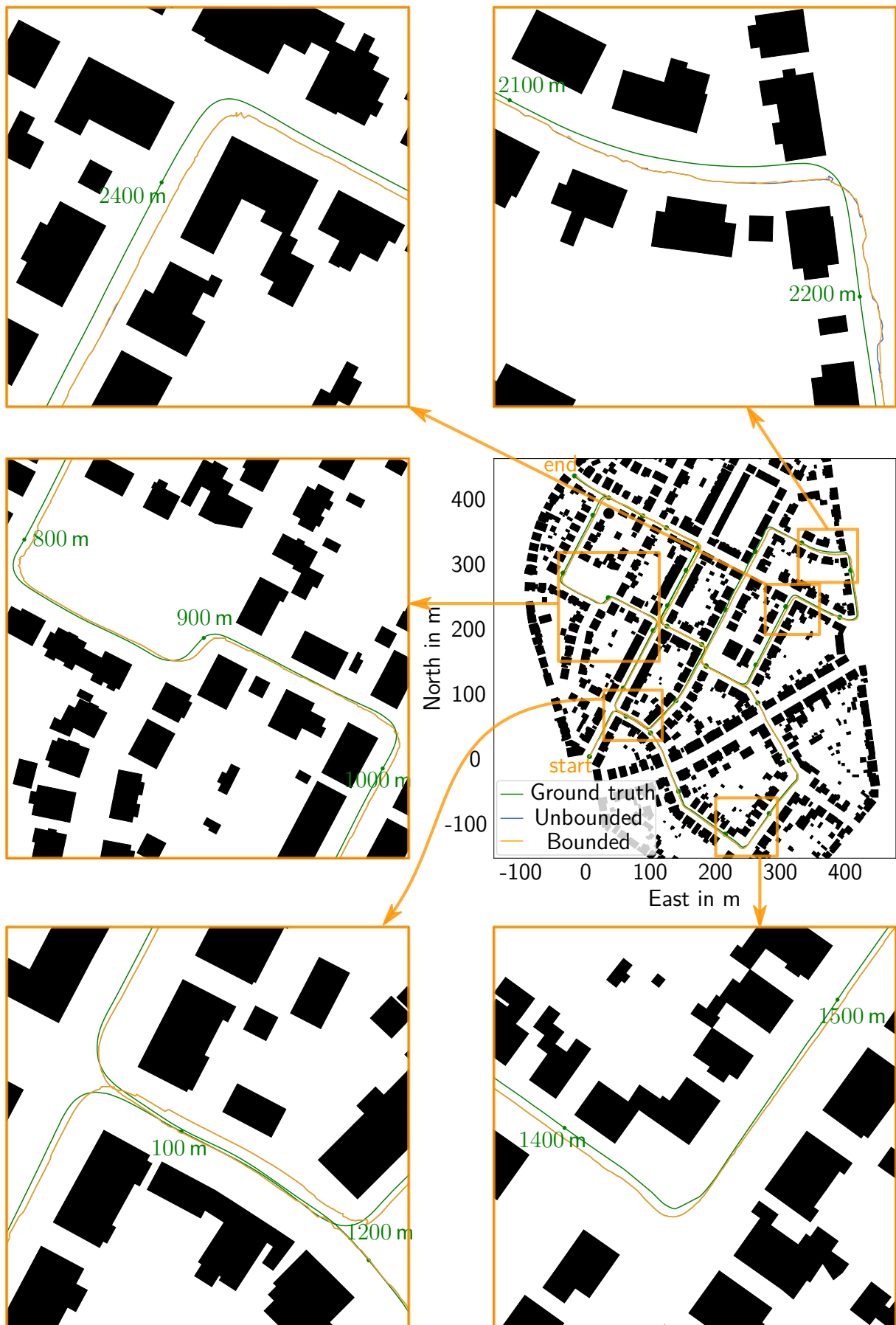
Figure 8.33: 0027 trajectory overview and selected close-ups. The ground truth trajectory is green, our result is orange, and the unbounded optimization result is blue.
