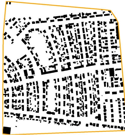
Figure 2.34: The convex polygon hull defines the border of the map. Black-filled polygons visualize the buildings. The map corresponds to the evaluation dataset KITTI 0018.
