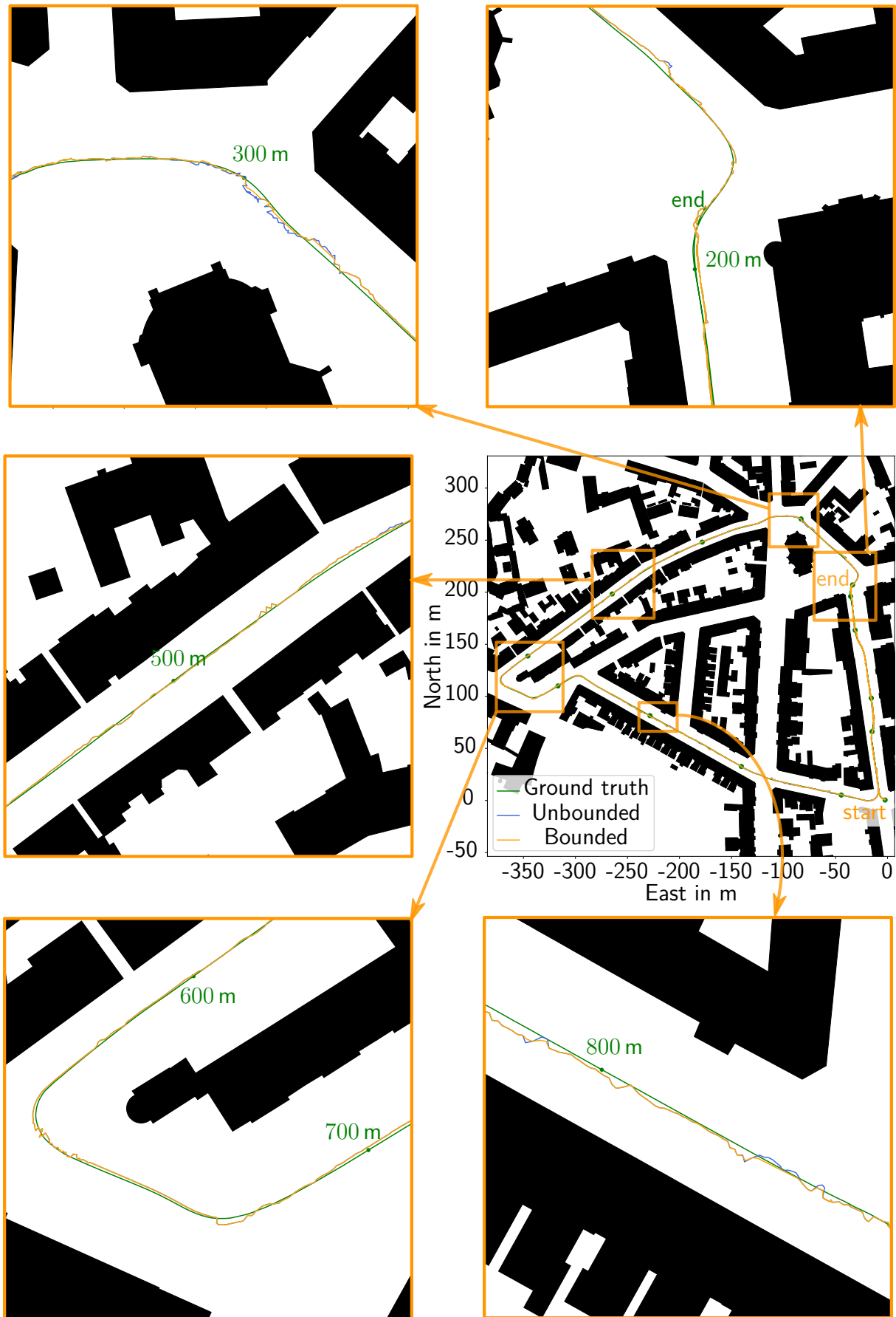
Figure 8.30: T_1 trajectory overview and selected close-ups. The ground truth trajectory is green, our result is orange, and the unbounded optimization result is blue.
