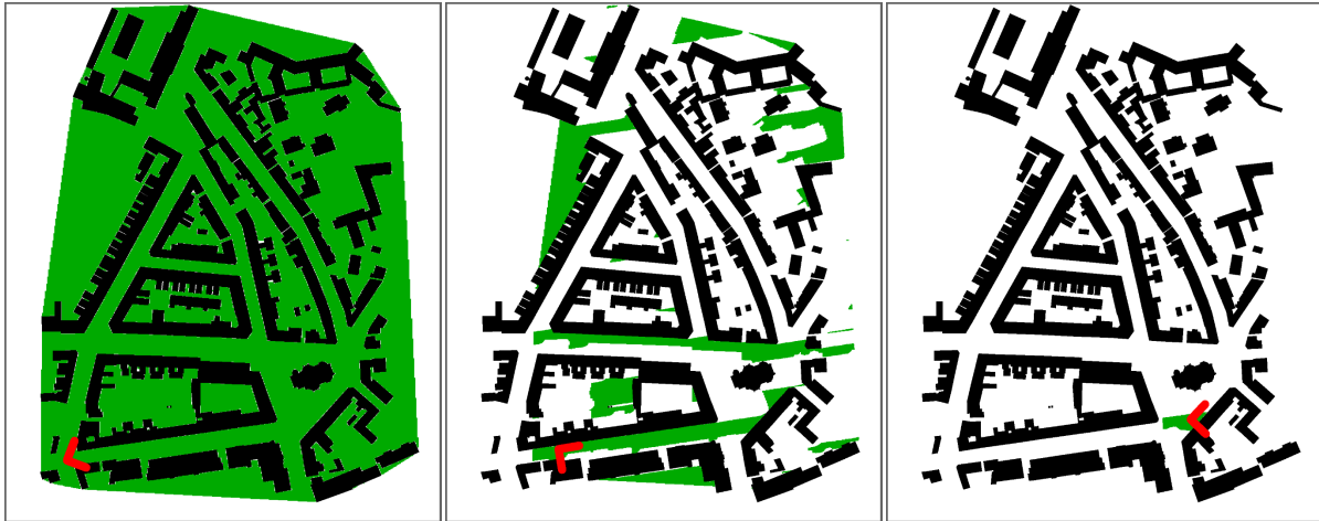
Figure 5.4: Localization sequence with correct initial orientation. The buildings are black and the set of all feasible vehicle positions is colored green. The ground truth pose is visualized red. The images show the localization result of a sequence starting on the left and ending on the right. The coarse localization is initialized in the left figure.
