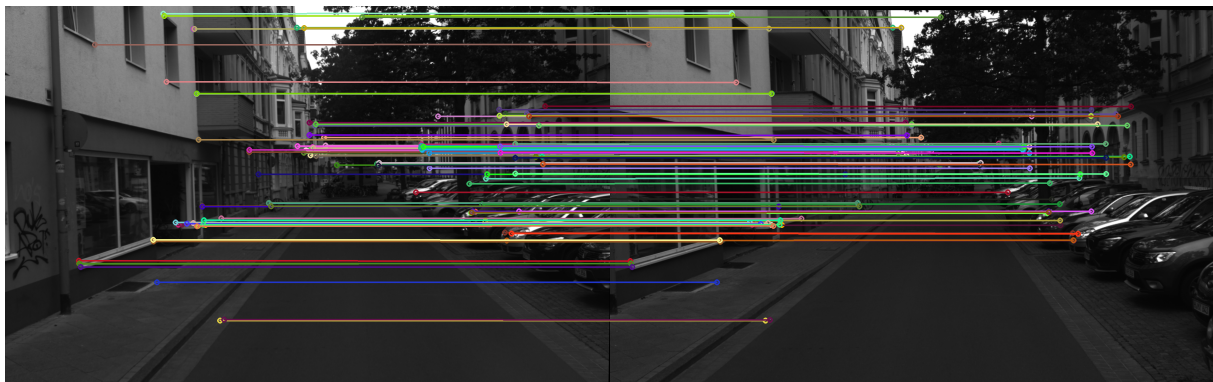
Figure 4.6: Feature matching in left and right images. Detected and tracked ORB-features in the left and right images are matched based on the binary BRIEF descriptor. Matched features are highlighted with the same color, and a connection line indicates their correspondence. Since we use stereo-rectified image pairs, the epipolar lines are horizontal. That is why the corresponding features in the left and right images are on the same image row.
