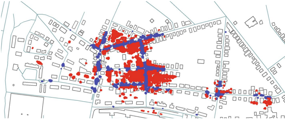
Figure 3.1: Pose candidates in a building map-based localization. The blue dots mark the valid and the red invalid candidates. [78]
