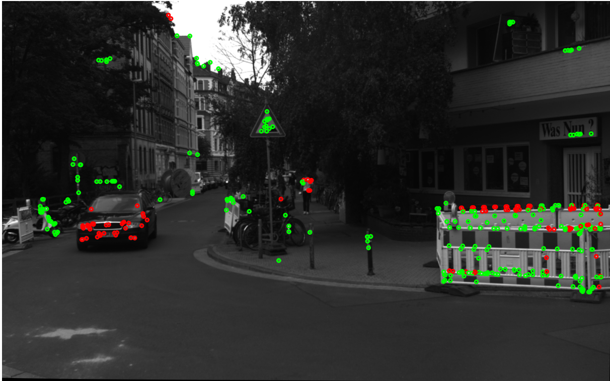
Figure 8.7: Outliers are detected and deleted by the robust windowed bundle adjustment. Successfully tracked features in the window that are detected as invalid due to high residuals in the windowed bundle adjustment are colored red, and good features that are permitted for the interval-based odometry computation are colored green.
