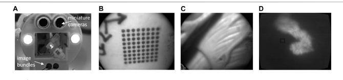
FIGURE 7 | (A) the µRALP endoscope tip with integrated dual imaging system (Tavernier et al., 2017). (B) and (C) white-light images acquired at 600 fps. (D) Fluorescence image acquired with the same imaging bundle.
