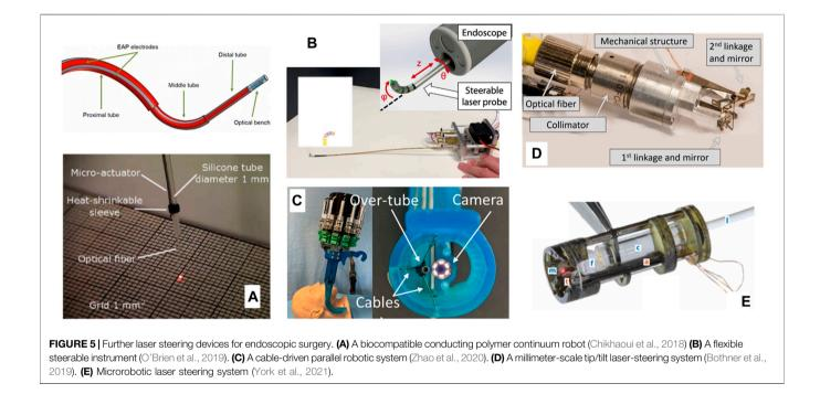
able to steer a laser beam using two optical wedges controlled by miniature piezoelectric motion systems, achieving a device that was 5 cm long by 17 mm diameter.
