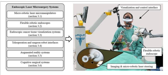
FIGURE 2 Core technologies of endoscopic laser microsurgery systems reviewed in this paper. These technologies can be integrated to create advanced robotic systems for delicate and high precision operations, such as demonstrated by the µRALP system for robot-assisted laser phonomicrosurgery shown on the right (Tavernier et al., 2017).
