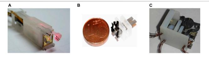
FIGURE 3 | Micro-robotic laser micromanipulators developed during µRALP. (A) Squipabot (Rabenorosoa et al., 2014). (B) PIBOT (Lescano, 2015). (C) Micro Agile-Eye (Lescano, 2015).
