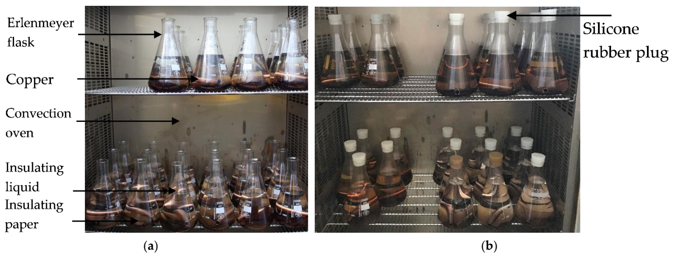
Figure 3. Thermally accelerated aging process of oil-paper insulation in a convection oven with Erlenmeyer flasks: (a) Open system; (b) Closed system.
