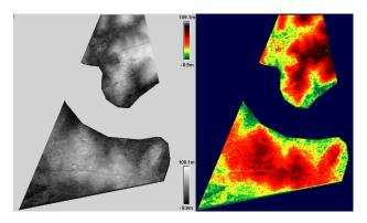
Figure 4. TSX SL DSM, grey and color coded presentation
