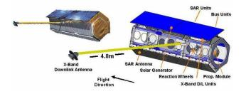
Figure 2. System components of TSX
