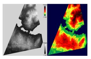
Figure 6. IKONOS DSM, grey value and color coded
