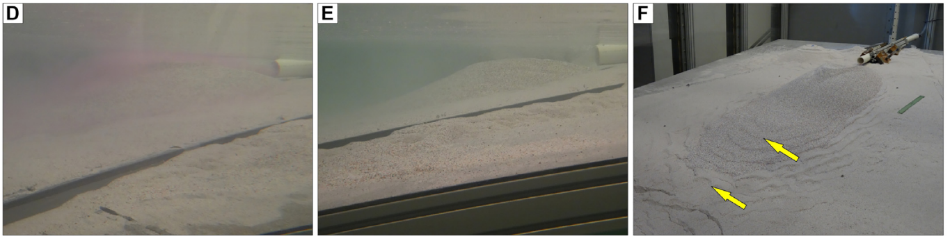
Formation of low-relief asymmetric bedforms on the lower slope of the mouth bar and beyond
