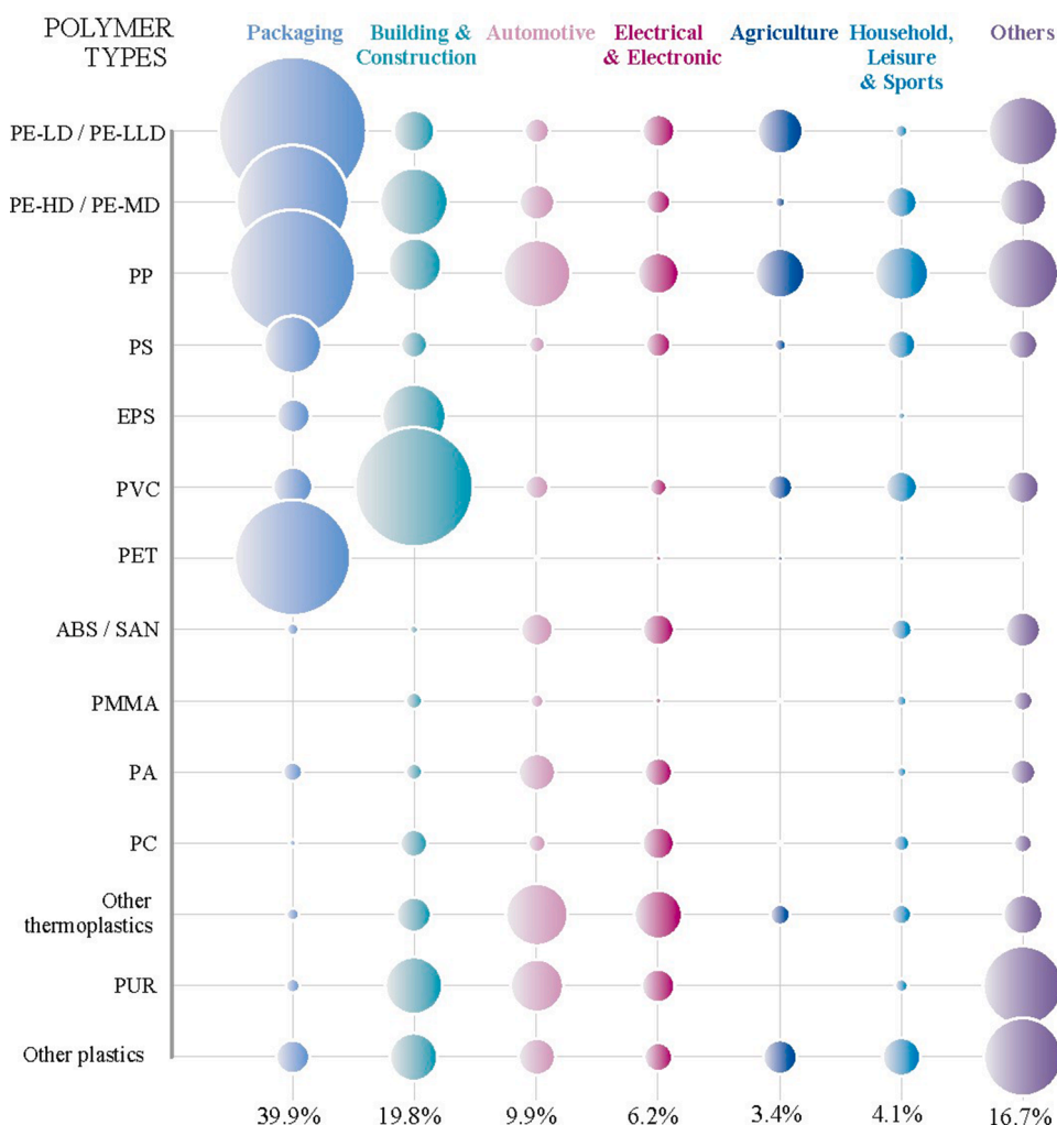
Fig. 5. Plastics demand by segments and polymer types in 2018. Total 51.2 mt data for EU, Norway and Switzerland [154]. Reproduced with permission from PlasticsEurope.
