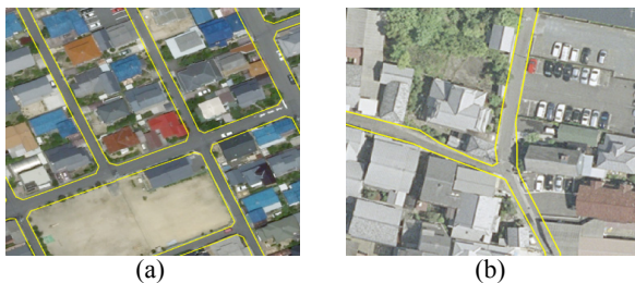
Figure 2. Two orthophotos superimposed by road edges (yellow). a) Buildings with coloured roofs and good contrast to the road; b) Buildings with a low contrast.
