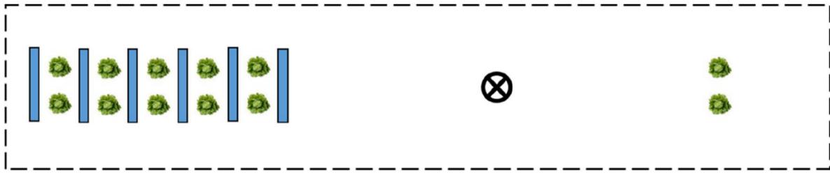
Fig. 2 Experiment setup phase II/II schematic. Flight trials in gauze tents (6 m × 1.2 m × 2 m) shown as scattered line, = ⊗ take-off point. Six LED panels (blue bars, control treatment without). Plant ratio
