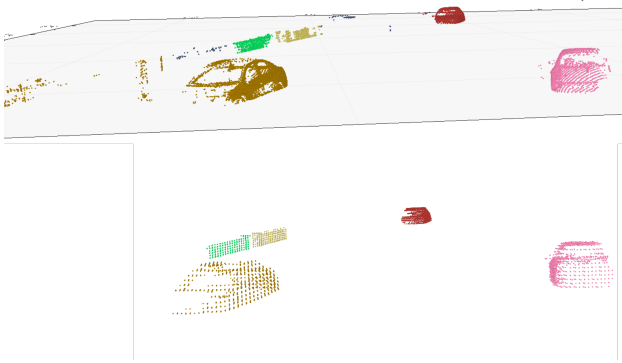
Figure 9. Visualization of the points labeled as car clustered and colored in single random color per cluster: before (upper part) and after region growing (lower part).
