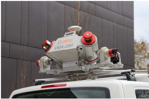
Figure 5. Riegl VMX-250 mounted on the top of the volkswagen T4.
