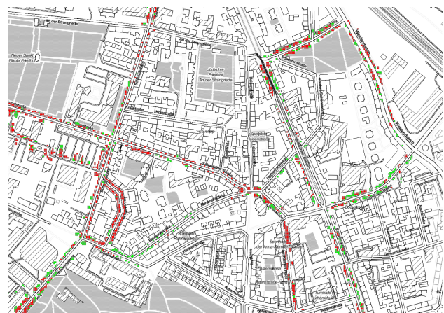
Figure 15. The availability of the space during the requested time period (12 am to 2 pm). Green cells encode free, red cells occupied space (basemap: Stamen Maps).
