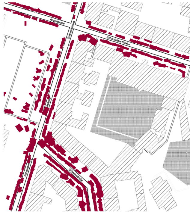
Figure 11. The extracted cars (red boxes) on top of a basemap (Stamen maps).
