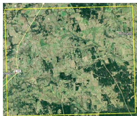
Figure 1. Google image of test site “Flat” Center: W95.91° N30.50°, 18km x 15km Height range: 72m – 139m, DSM spacing 29m / 86m Average multiple coverage for TDM90 = 2.7 and for AW3D30=3.8; influence of interpolation over 29m= 0.25m, over 86m= 0.53m (terrain roughness)
