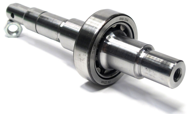
Fig. 2 Hybrid shaft (total length of 146.5 mm) with mounted cylindrical roller bearing after testing
