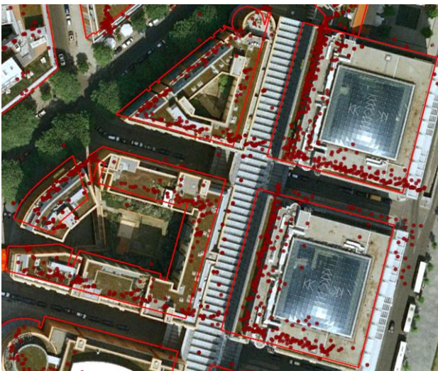
Figure 4. Outlines and PS before application of the estimated shift for a small part of the test site. The offset between both datasets is clearly visible.
