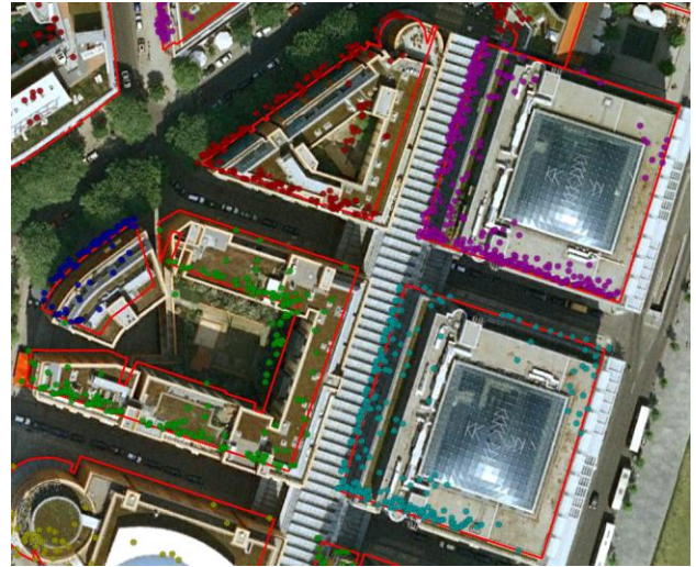
Figure 5. Outlines and PS after the PS set has been shifted. The alignment is clearly visible. The assignment to the buildings is indicated by the colours.
