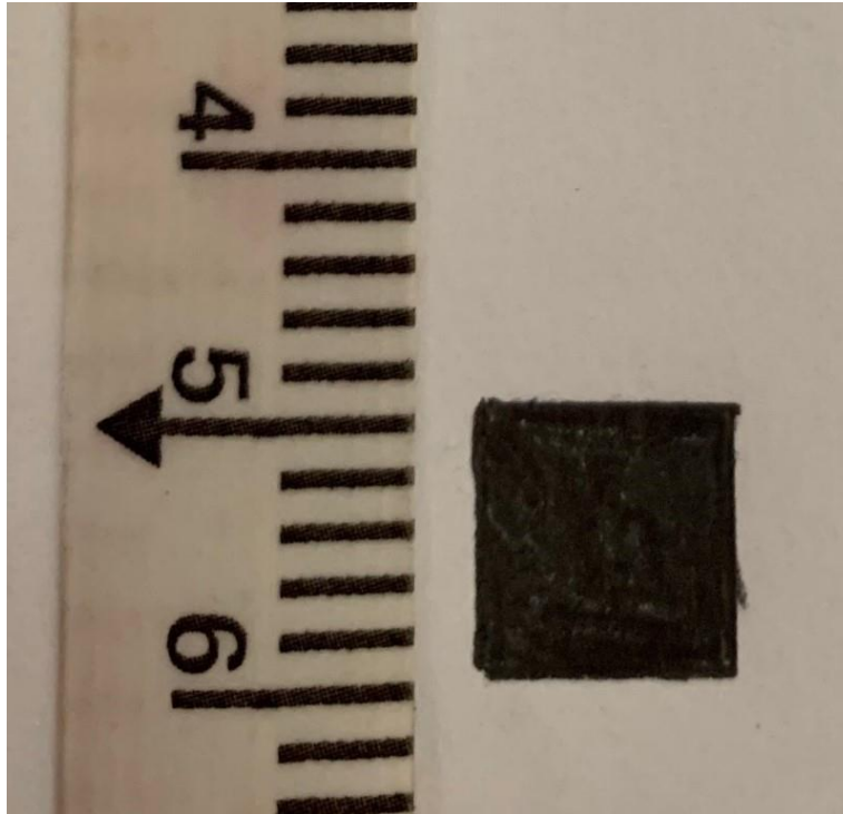
Fig. 3.10: Validation of Matlab Image processing by measuring 1 cm 2 black area
