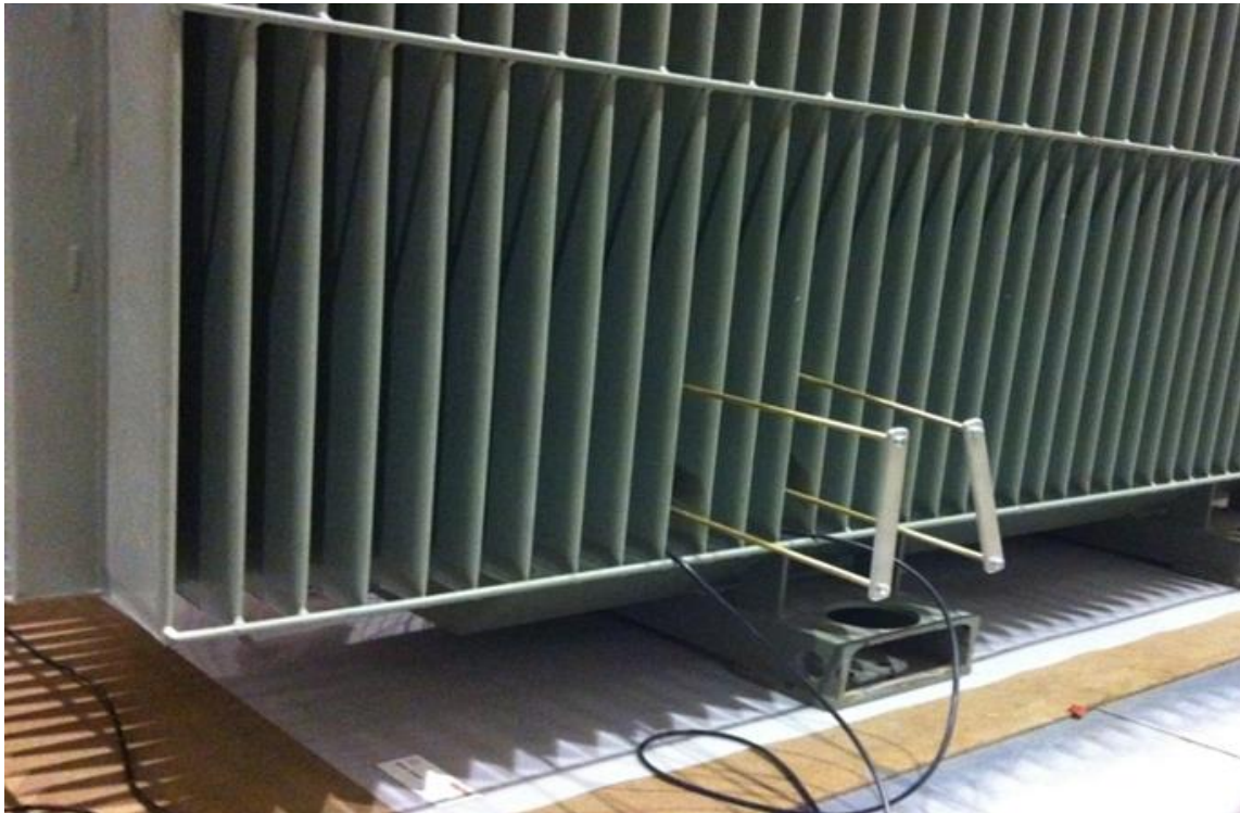
Fig. 0.1: Part of a transformer with special casing of the AE sensors to install in large dimension of cooling system
