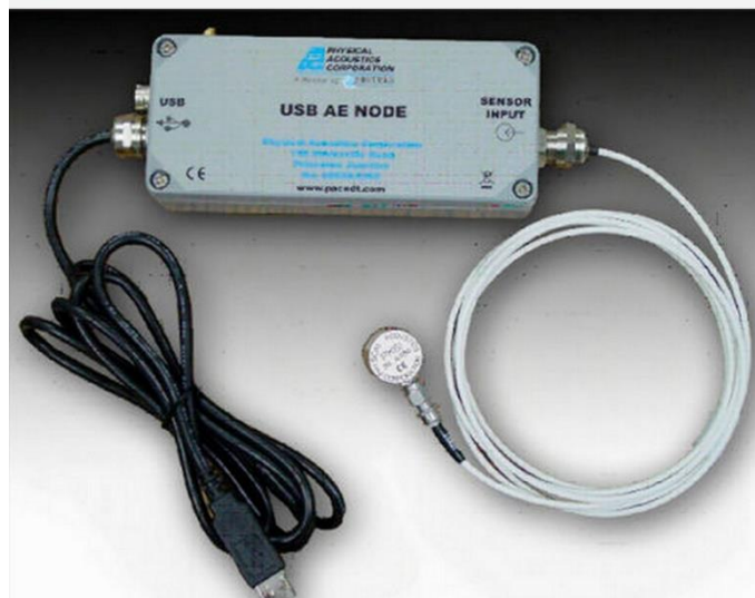
Fig. 2.10: Physical Acoustic DSP device with connected acoustic sensor [79]
