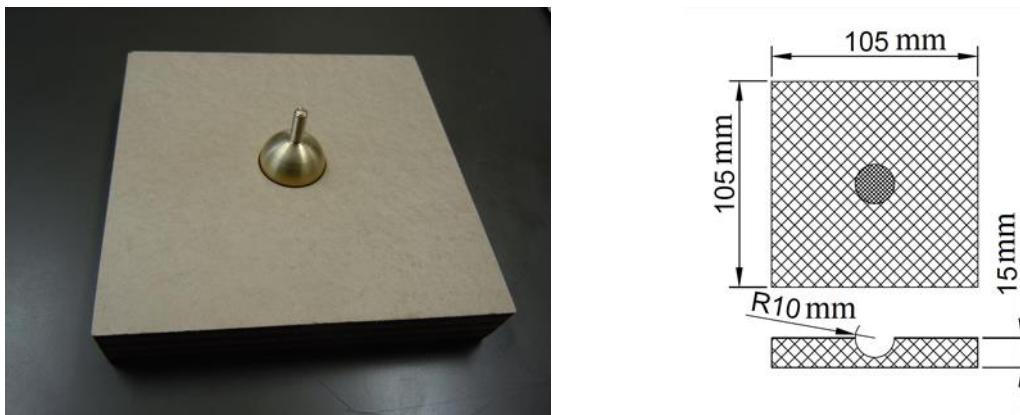
Fig. 4.10: 15 mm thickness pressboard with 20 mm electrode diameter inside the hole at the centre
