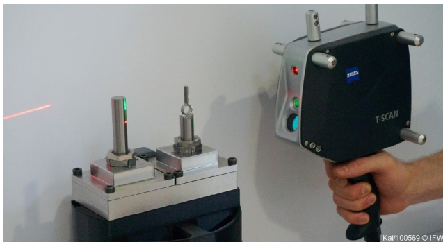
Fig. 4. Handheld laser scanner
