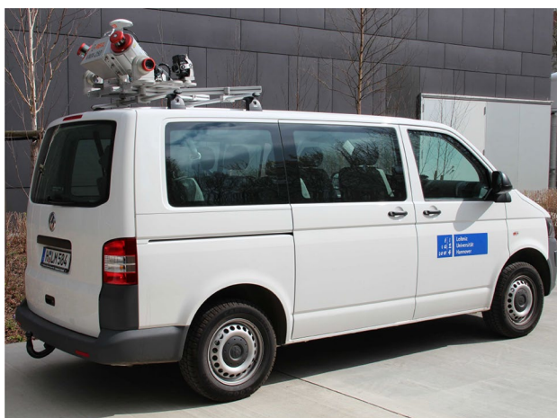
Fig. 1 Measurement van with Riegl VMX-250
