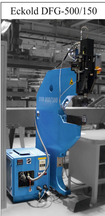
Fig. 2 Clenching press of the company Eckold (down) and the company TOX (up); the used clenching tool system of the company BTM (down) and the company TOX (up)
