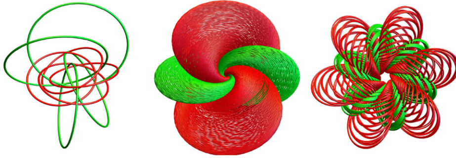
Figure 1. Electric (red) and magnetic (green) field lines at t = 0 with four fixed seed points. Left: (0; 0, 1)_I configuration. Center: (\frac{1}{2}; -\frac{1}{2}, \frac{3}{2})_R configuration. Right: (1; 1, 2)_I configuration. More self-knotted field lines start appearing with additional seed points in the simulation.
