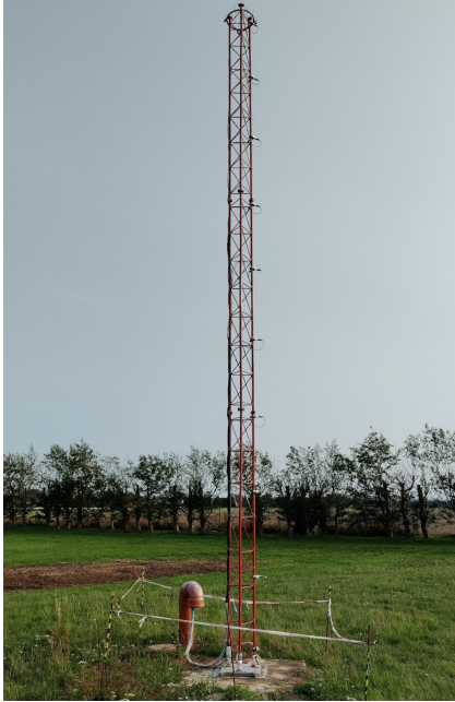
Figure 5.1: Girder-mast structure located at the outdoor facility. Acceleration sensors are arranged in a biaxial setup along one of the three legs.
