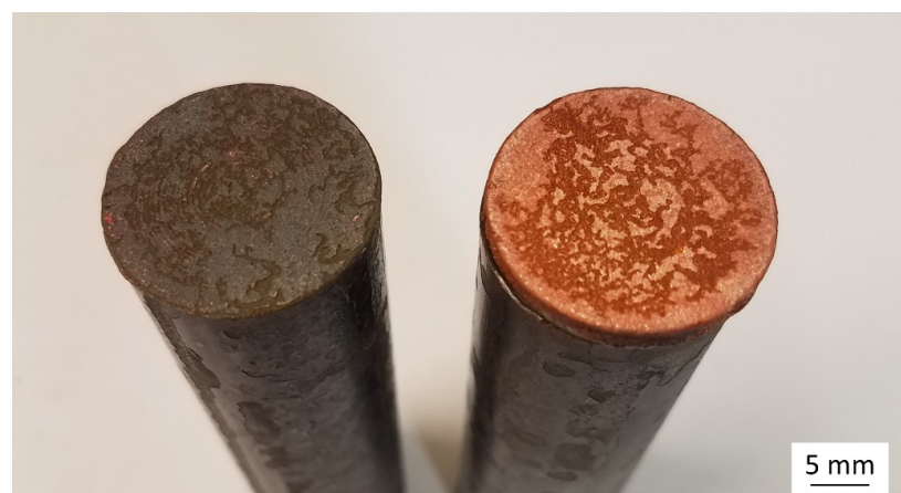
Figure 5. Representative adhesive tensile stamp with adhesive failure after a tensile strength test.
