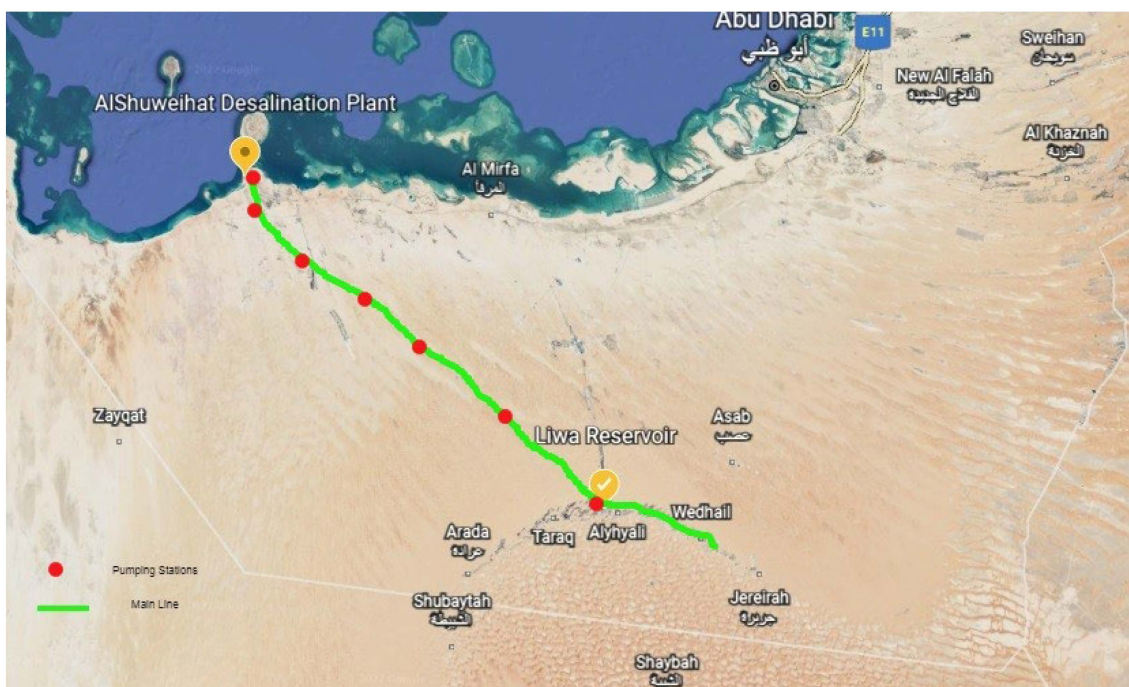
Figure 1. A schematic for part of TRANSCO Water Transmission Network showing AlShuweihat to Liwa transmission line.
