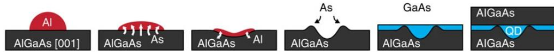
Figure 1. 14. Sketch of local droplet etching and nanohole infilling. Adapted from Ref.[96] https://www.nature.com/articles/ncomms15501 . Licensed under CC BY 4.0.
