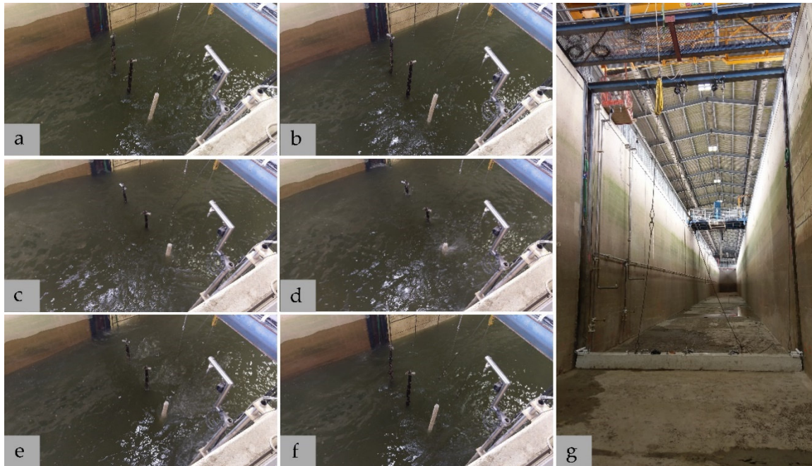
Figure 25: (a - f) Depiction of a single wave ( H = 0.8 m, T = 6 s) passing two blue mussel ( Mytilus edulis ) specimen and the SM 1 surrogate. The wave peak (d) passes the live blue mussel dropper lines, and the surrogate, with a length of 2.0 m each, which were mounted to stainless steel wires connected to a concrete block at the bottom and a steel beam at the top of the flume (g) in a distance of approximately 97 m from the wave machine.
