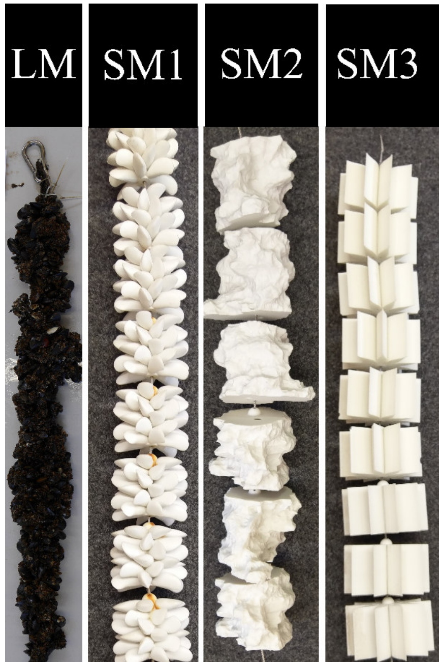
Figure 11: Live mussel dropper line (LM) next to surrogate mussel dropper line 1 (SM 1), surrogate mussel dropper line 2 (SM 2) and surrogate mussel dropper lines 3 (SM 3).
