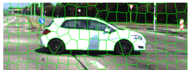
Figure 4. Superpixels. Typical oversegmentation of a car.
