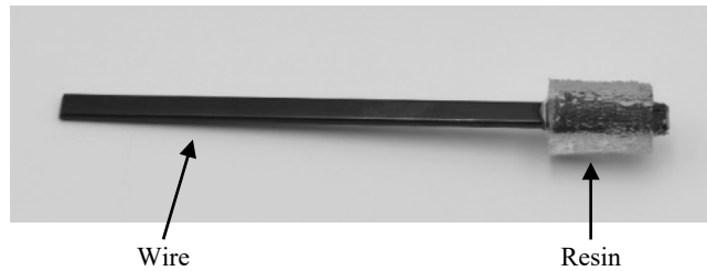
Figure 5: Finished wire sample with cured resin
