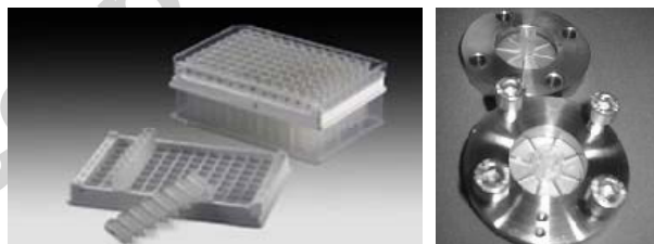
Figure 1: 8-strip membrane adsorbers placed on 96-well plates are used in a centrifuge (left), LP-15 Membrane adsorber test systems can be used for analyzing performance in an up-scale to milliliters (right)
