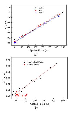
**Figure 7.** Response of the 1D FCS sample (a) to applied force as well as the response of the 2D FCS to applied longitudinal and normal forces (b).
