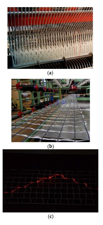
**Figure 2.** Wrap knitting machine that can simultaneously process alkaline-resistant glass and optical glass fibers ( $\mathbf{a}$ ) and, hence, which was applied to fabricate the fiber optic crack sensor ( $\mathbf{b}$ , $\mathbf{c}$ ).
