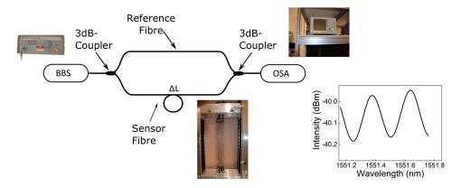
**Figure 5.** Developed fiber optical MZI to evaluate and characterize the force transfer between the carbon structure and the optical fiber of the FCS.
