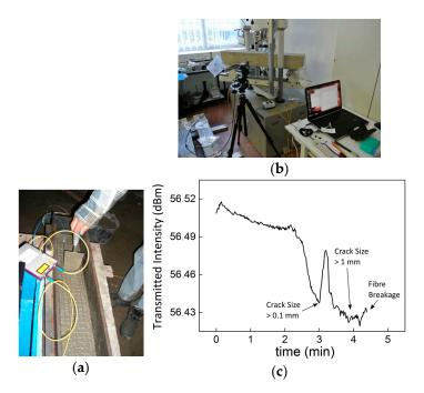
**Figure 3.** Embedding the sensor in a concrete block (a) and experimental set-up (b) for the evaluation of the fiber optic crack sensor performance (c).
