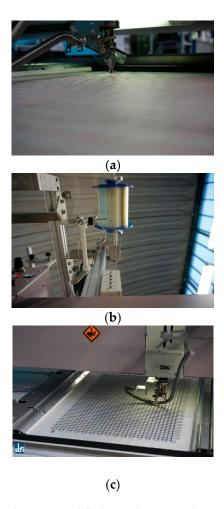
**Figure 4.** Embroidery machine that was modified in order to simultaneously process carbon filaments and optical fibers. The modification included the development of an appropriate embroidery needle (a) and a mechanism to auto-track the optical fiber during fabrication of the FCS (b) to process the carbon filaments and optical glass fiber simultaneously on a nonwoven substrate made of PVA (c).
