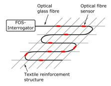
**Figure 1.** Sketch of a textile reinforcement structure that is functionalized with fiber optic sensors in order to monitor important SHM parameters. The textile reinforcement structures are designed so that they can act as both sensing and strengthening mechanism.
