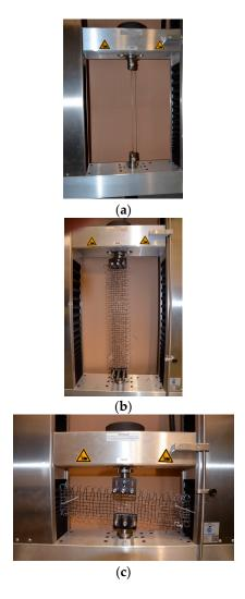
**Figure 6.** Functionalized 1D and 2D FCSs mounted to the tensile testing machine MFC T3000 in order to evaluate the force transfer between the carbon filament and the optical fiber (a) as well as the sensitivity to longitudinal (b) and normal (c) forces.
