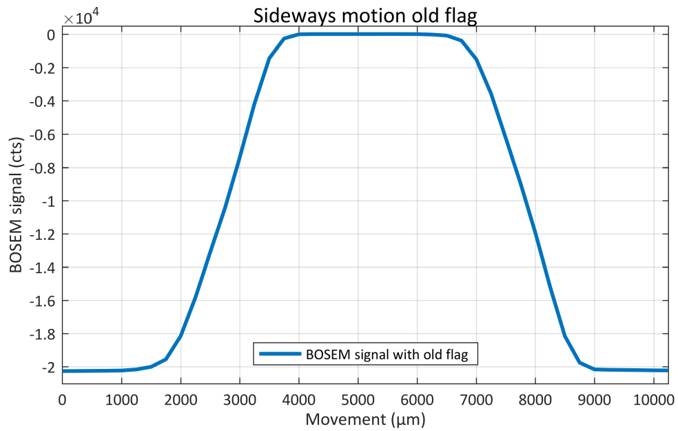
Figure 4.36: The power measured by the BOSEM as a function of the sideways flag position. In this plot, an old flag was used, having a width of 5 mm.
