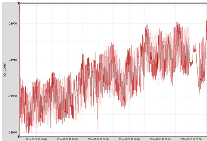
Figure 4.35: A measurement of the BOSEM output over 12 d. The short-term fluctuations correspond to temperature changes in the lab, the long-term drift is due to a slow degradation of the BOSEM sensor.
