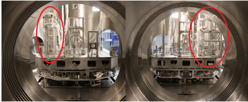
Figure 3.14: The two suspension cages of the reference cavity. On the left, the end mirror of the triangular cavity, located on the south table, is visible. On the right, input and output mirrors, making up the short arm of the cavity, are visible on the central table. The separation is 10 m.
