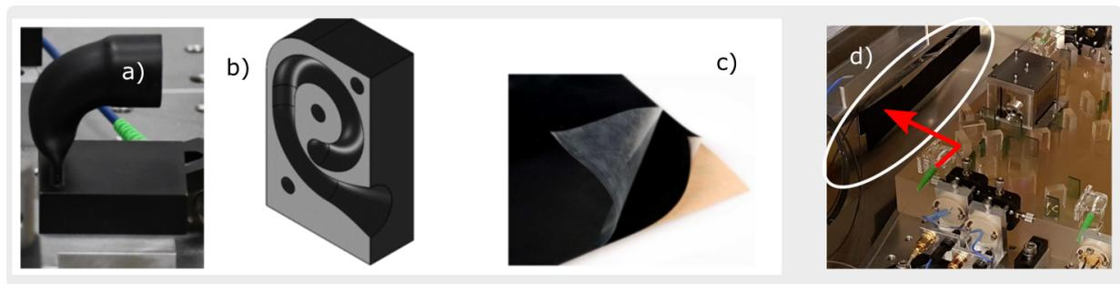
**Fig. E.1.:** Three different types of beamdumps, picture based on [Jes22]. a) AEI standard beamdump, b) textitspiral Beam Dump by M. Perreur-Lloyd, c) black foil from the company *Acktar*. d) Foil attached to the thermal shield and beam path sketched from *fios1* reflected by *att1*.
