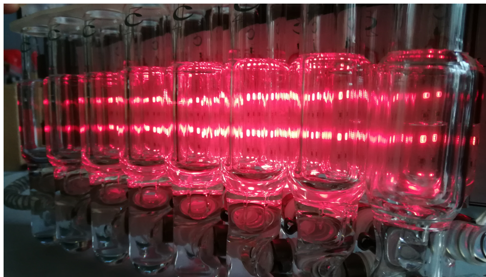
Figure 2.38 Reactor array of the ASW 2000P with one half of the photoreactor array installed.
