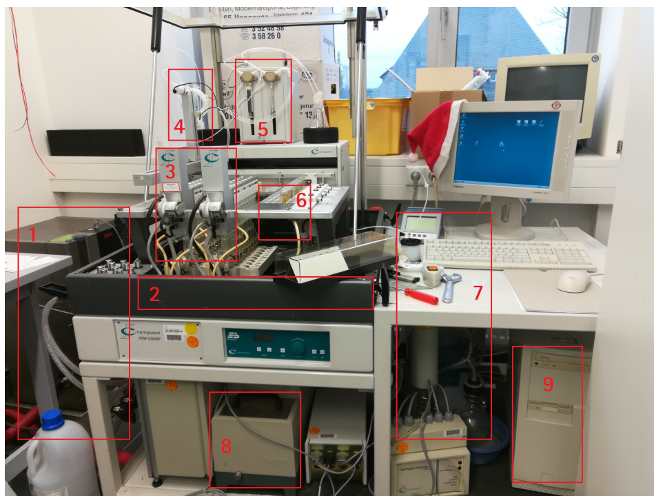
Figure 2.1 Photograph of the ASW 2000P parallel synthesizer. 1: Reaction thermostat. 2: Vortex table. 3: Reactor blocks. 4: Robotic arm. 5: Syringe pumps. 6: TLC chamber, reagent rack. 7: Vacuum system. 8: Reflux thermostat. 9: Control station.
