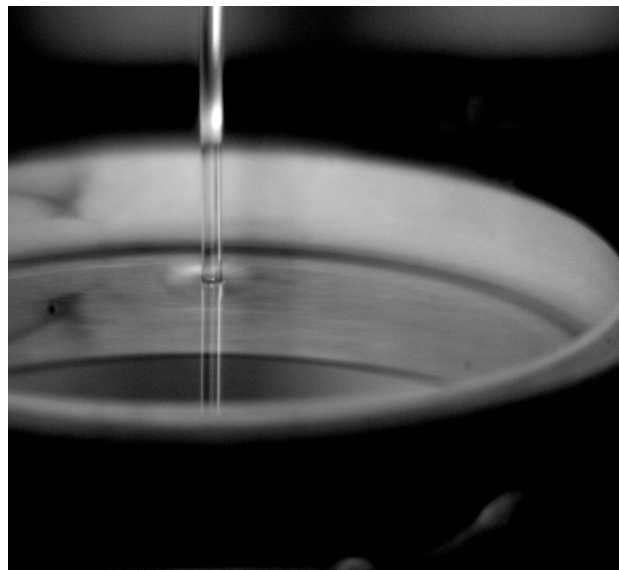
Figure G.0.2: Corning-7980-0F glass window spliced to the PLMA-EYDF-25P/300-HE fiber with a \text{CO}_2 laser.
