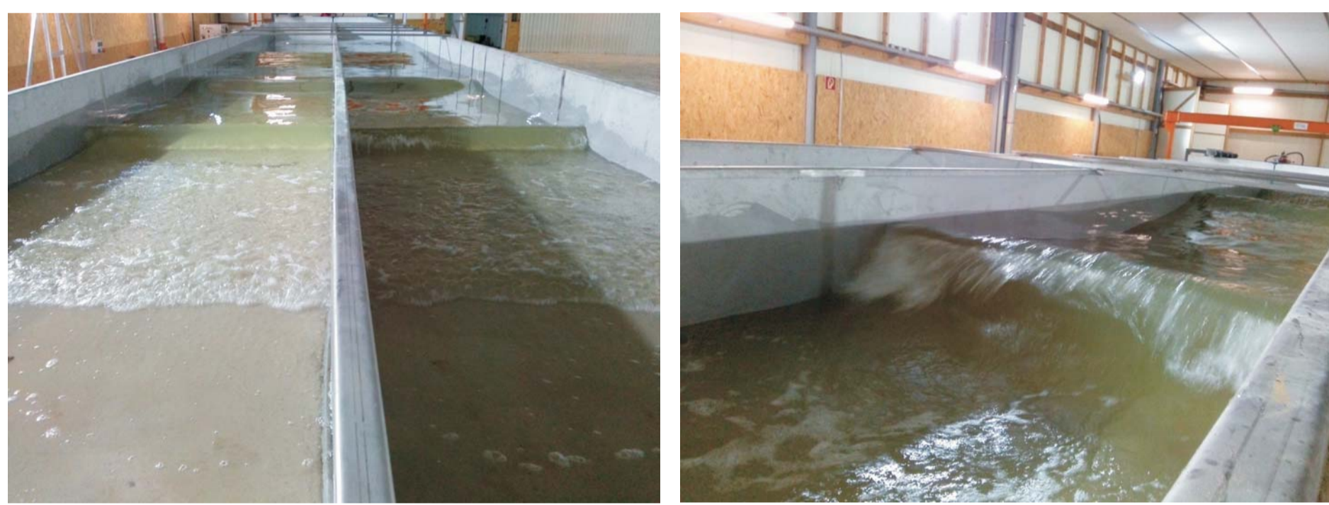
Fig. 1: Wave flume construction as a twin flume with one wave paddle
