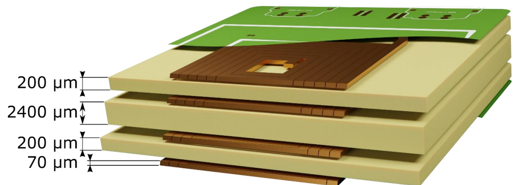
Figure 1. Schematic sectional view of the Square PCB transformer, showing the layer structure.
