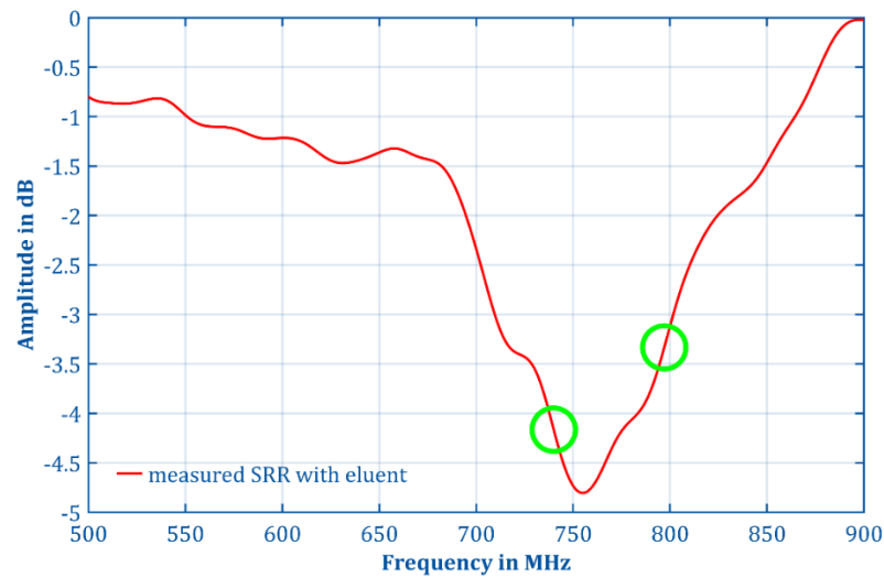
Figure 10. Measured transmission response (red) of the CaSRR loaded with the eluent and recorded with the new readout electronics. The resonance frequency was 755 MHz for the used eluent consisting of 25% ultrapure water and 75% acetonitrile, and the attenuation was -4.806 dB. The green circles mark the optimum excitation frequencies at 740 MHz and at 797 MHz for highest sensitivity regarding the detection of resonance frequency shifts.
