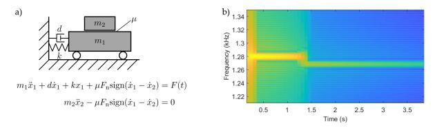
Figure 3: a) Dual mass model and equations of motion; b) STFT result after impact excitation from numerical time integration
