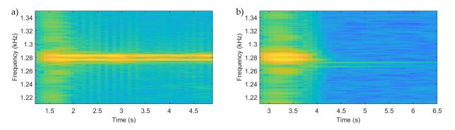
Figure 2: STFT results after impact excitation: a) unfilled pipe ; b) pipe filled with a small amount of sand
