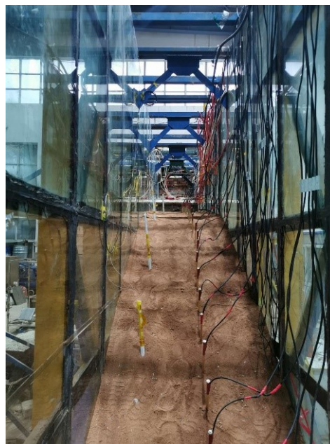
Figure 4. A picture of the landslide model built indoors, from a frontal view: the model was 1.5 m (height) * 0.8 m (width). The water content sensor is inside the landslide body (not visible; the actual water content sensor is shown in Figure 6a).
