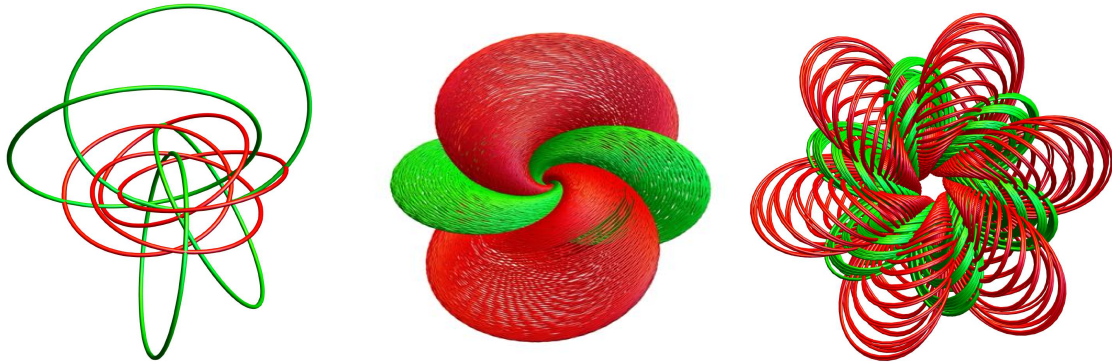
FIGURE 5.1: Electric (red) and magnetic (green) field lines at t=0 with 4 fixed seed points. Left: (j; m, n) = (0; 0, 1)_I configuration, Center: (j; m, n) = (\frac{1}{2}; -\frac{1}{2}, \frac{3}{2})_R configuration, Right: (j; m, n) = (1; 1, 2)_I configuration. More self-knotted field lines start appearing with additional seed points in the simulation.
