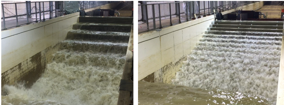
Figure 4.11: Residual layer of water on stepped revetments as next wave approaches. (a) Configuration 1 with S_h=0.50\text{m} and (b) Configuration 2 with S_h=0.17\text{ m}
