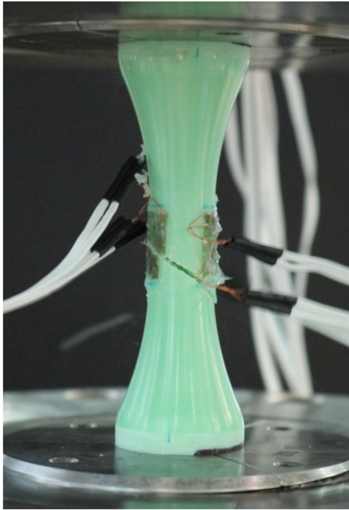
Fig. 12. Typical fracture observed in the biaxial tests with an initial strain rate ratio of \dot{\epsilon}_0/\dot{\gamma}_0 = 1/4 .
