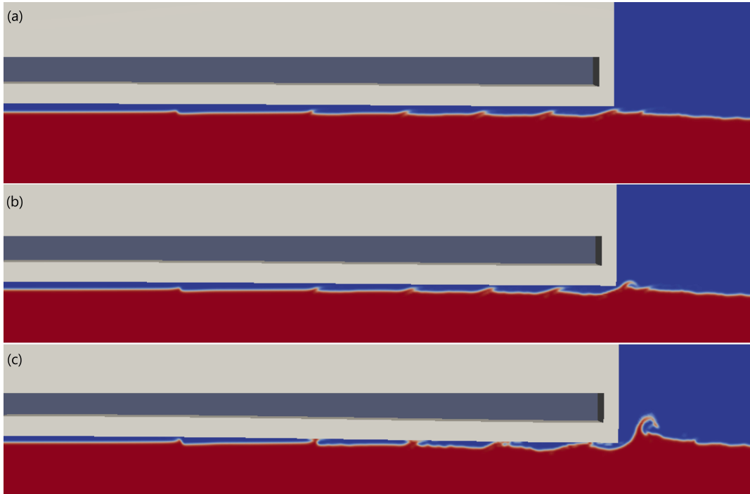
Figure 3.10: Formation of air cushion at the beginning of impact in numerical model. The scenes are from (a) 2 ms before the impact, (b) at the time of impact, and (c) 8 ms after the impact.
