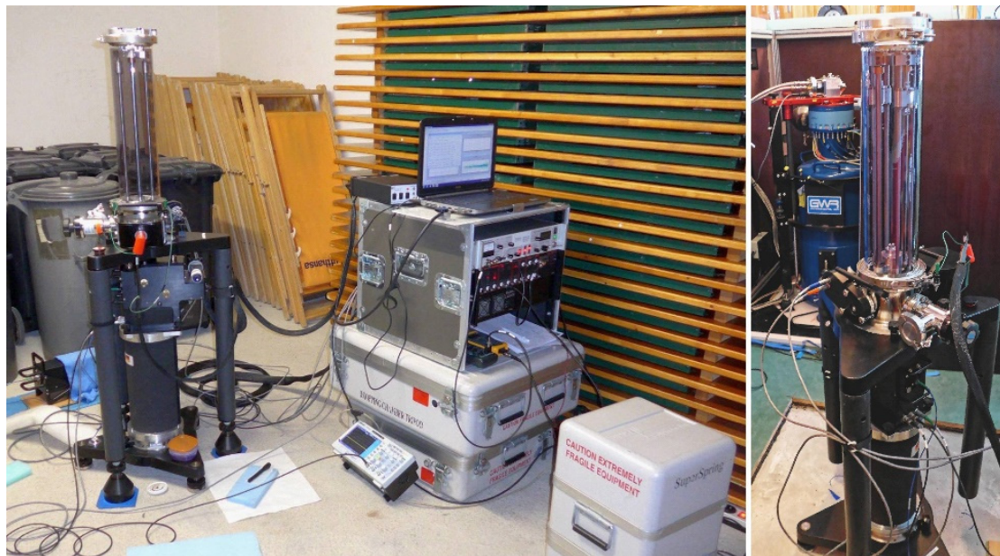
Figure 3. (left) Absolute gravimeter FG5-220 with control electronics at the site Wank Berg in 2019; (right) FG5-220 operating close to the superconducting gravimeter OSG#052 at Zugspitze.
