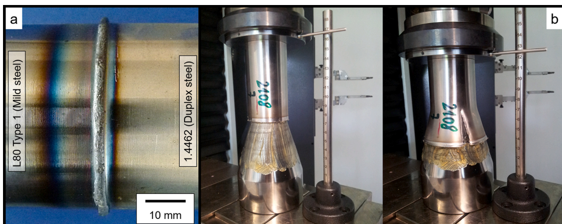
Fig. 5. Colouring of the welds indicating the difference in heat dissipation of the two materials (a); test set-up used for expansion testing of the pipe joints (b).
