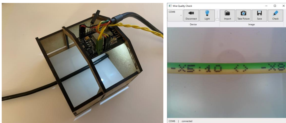
Figure 3: Photo of the hardware (left) and software (right) prototype to identify the markings.
