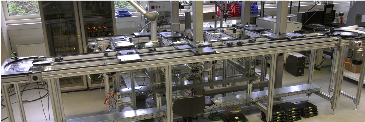
Figure 3: Test setup with double belt conveyor
