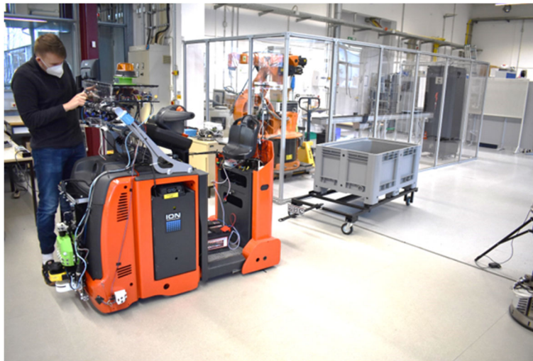
Figure 1: Autonomous tow truck for the exemplary realisation of the hybrid metric
